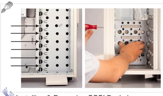
Installing & Removing SCSI Backplane Boards
